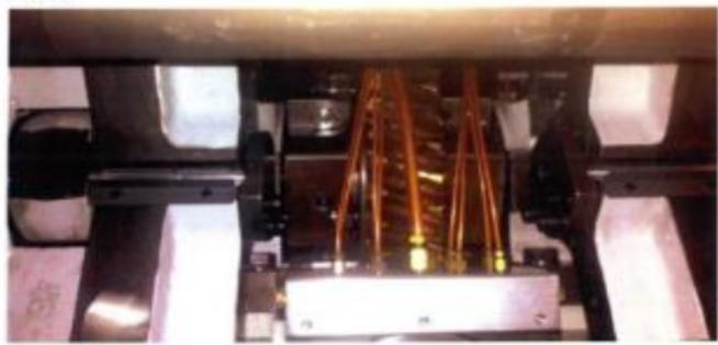
The position of the cam support bracket was shifted which was caused by a heavy impact and could lead to the damage of the worm gear shaft. The consequence of the shaft damage could lead to shorter life span of the machine, shaft breaks during high cutting pressure and improper mechanical movement of the machine.
